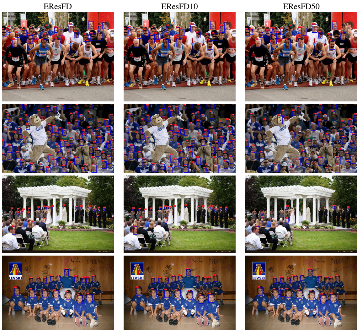
Figure 5. Visualisation of face detection examples using the original EResFD model (first column) and its pruned variants, EResFD10 (second column) and EResFD50 (third column). As with our EXT D examples (Figure 4), we see that in many cases, the model derived using the proposed approach with 10% pruning rate outperforms the original one in terms of detection performance.
